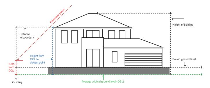
Recession plane calculated from the closest point to the boundary from the average original ground level
