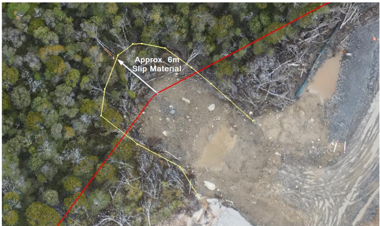
Figure 1: Red line is consent boundary. + is consent boundary peg, original and moved. Yellow line marks slip extent.
