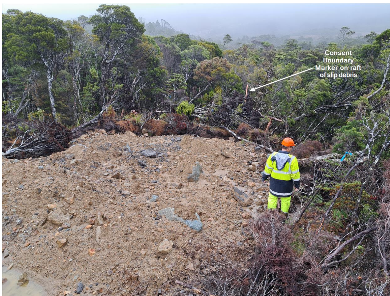
Figure 4: Weathered rock/mud backed-up behind the leading edge of the slip.
